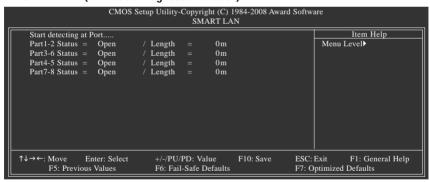
This motherboard incorporates cable diagnostic feature designed to detect the status of the attached LAN cable. This feature will detect cabling issue and report the approximate distance to the fault or short. Refer to the following information for diagnosing your LAN cable:
