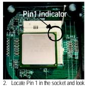
for a (golden) cut edge on the CPU upper corner. Then insert the CPU into the socket.
