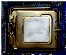
Fig. 1 Please apply an even layer of CPU cooler paste on the surface of the installed CPU.
