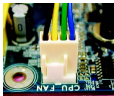
Fig. 6 Finally, please attach the power connector of the CPU cooler to the CPU fan header located on the motherboard.
