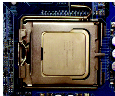
Fig. 4 Once the CPU is properly inserted, please replace the plastic covering and push the metal lever back into its original position.
