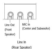
After install onboard audio driver, you may connect speaker to Line Out jack, micro phone to MIC In jack.
