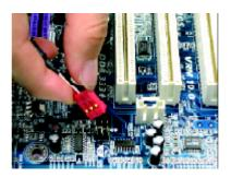
Connect co-axial or optical output to the SPDIF decoder.
