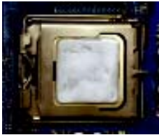
Fig. 1 Please apply an even layer of heatsink paste on the surface of the installed CPU.
