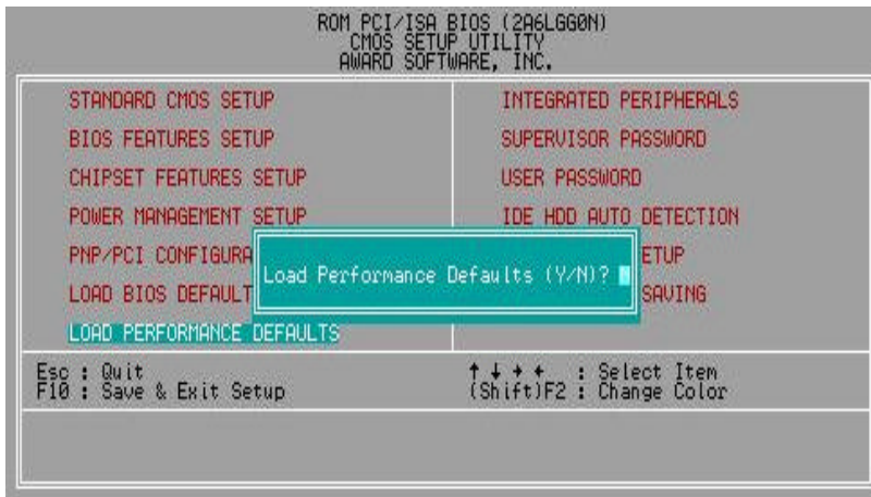
Figure 4.8: Load Performance Defaults
