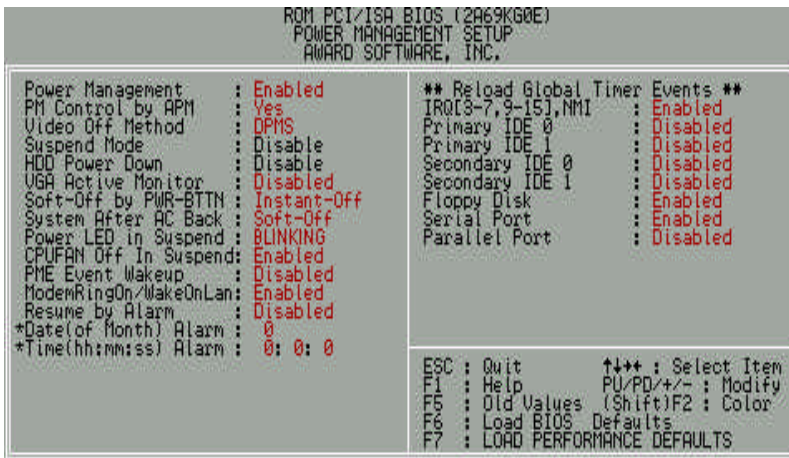
Figure 4.5: Power Management Setup
