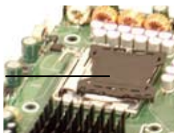
Plastic cap is released from the load plate if CPU properly installed.
