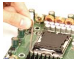
CPU in the CPU socket
