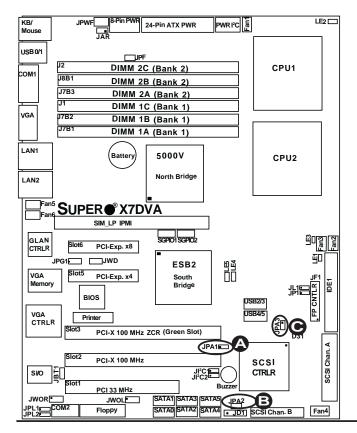
A. SCSI EnabledB. CH. A Termination EnabledC. CH. B Termination Enabled
