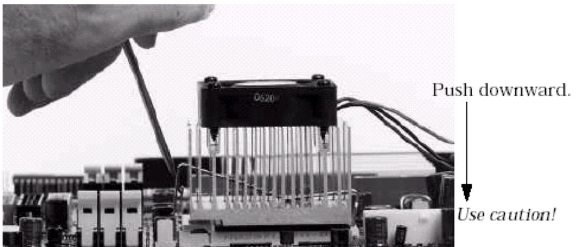
4. The fans power connector should be connected to CPUFAN1.
