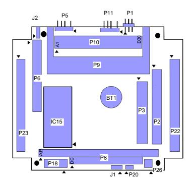
Figure 1. MICRON PCB - Top View Showing Connector Positions. Pin 1 of each connector is indicated by an arrow.
