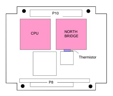
Figure 2. MICRON PCB - Underside View Showing Hot Devices and Temperature Sensor.
