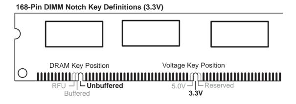
The notches on the DIMM module will shift between left, center, or right to identify the type and also to prevent the wrong type from being inserted into the DIMM slot on the motherboard. You must ask your retailer the correct DIMM type before purchasing. This motherboard supports four clock signals.
