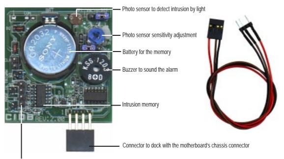
Two switch connectors to detect intrusion by chassis mounted micro switches
