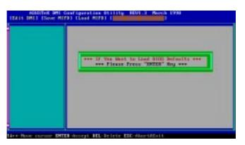
You can load the BIOS defaults from a MIFD file and can clear all user modified and added data. You must reboot your computer in order for the defaults to be saved back into the Flash BIOS.
