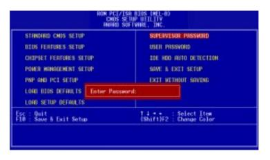
To implement password protection, specify in the "Security Option" field of the BIOS Features Setup screen when the system will prompt for the password. If you want to disable either password, press <Enter> instead of entering a new password when the "Enter Password" prompt appears. A message confirms the password has been disabled.
