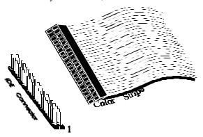
J10 is a 40-pin dual-inline berg that connects an IDE drive to the primary onboard IDE connector. This motherboard supports IDE Modes 0, 1, 2, 3, and 4, IDE prefetch, LBA (Logical Block Address) mode, high capacity drives (over 528 MB), 32-bit data transfer, and fast IDE transfer. These IDE features are configured in Peripheral Setup in the WINBIOS Setup utility.
