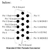
Standard VGA Connector The pinout for the standard female DB15 VGA connector is shown below:
