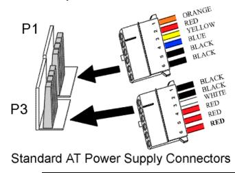
**Power Connector Keys** The power connectors are keyed to prevent incorrect installation. The keys on the connector must be cut to fit on some power supplies, as shown below.
