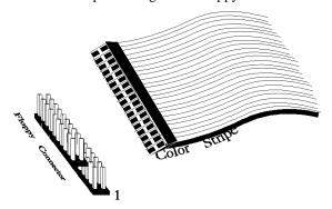
The motherboard supports up to two 720 KB, 1.44 MB, or 2.88 MB 3<sup>1</sup>/<sub>2</sub>" drives and 360 KB and 1.2 MB 5<sup>1</sup>/<sub>4</sub>" drives. The connecting cable is a 34-pin ribbon connector with two 34-pin edge connectors for attaching the floppy disk drives. There is a small twist in the cable between the floppy connectors. The last (end) connector should be connected to floppy drive A:.
