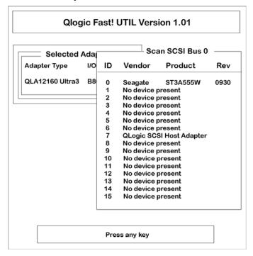
**Scan Disk Utility Screen** You can use the Scan Disk Utility screen to perform a low-level format or verify the disk media for a disk device. The following information for the selected SCSI bus displays:
