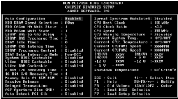
Figure 6-4: The Chipset Features Setup screen.
