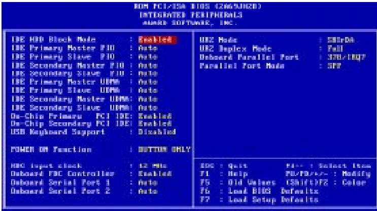
Figure 6-7: The Integrated Peripherals screen.
