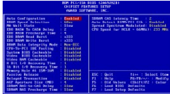
Figure 6-4: The Chipset Features Setup screen.
