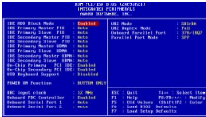
Figure 6-7: The Integrated Peripherals screen.
