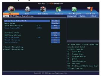
Extreme Memory Profile (X.M.P.) (Note), System Memory Multiplier, Memory Frequency(MHz) The settings above are synchronous to those under the same items on the Advanced Frequency Settings menu.
