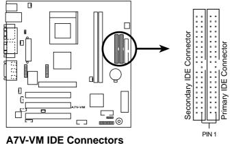
**NOTE:** Orient the red markings (usually zigzag) on the IDE ribbon cable to PIN 1.
