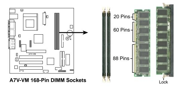
The DIMMs must be **3.3V Unbuffered** for this motherboard. To determine the DIMM type, check the notches on the DIMMs (see figure below).
