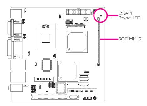
The system board is equipped with 2 SODIMM sockets. SODIMM 2 is located on the component side of the board. SODIMM 1 is a 90° socket located beneath SODIMM 2.
