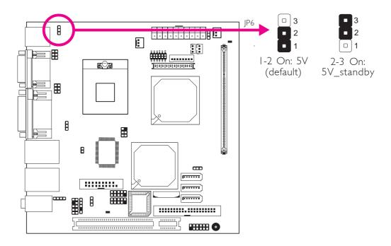
JP6 is used to select the power of the PS/2 keyboard/mouse port. Selecting 5V\_standby will allow you to use the PS/2 keyboard or PS/2 mouse to wake up the system.
