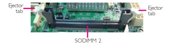
5. Note how the module is keyed to the socket. Grasping the module by its edges, position the SODIMM above the socket with the "notch" in the module aligned with the "key" on the socket. The key ensures the module can be plugged into the socket in only one way.
