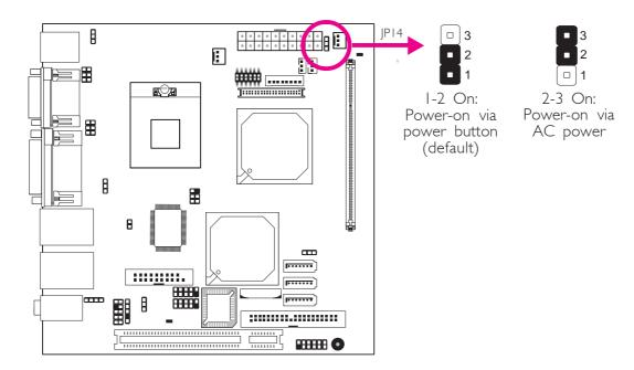
JP14 is used to select the method of powering on the system. If you want the system to power-on whenever AC power comes in, set JP14 pins 2 and 3 to On. If you want to use the power button, set pins 1 and 2 to On.
