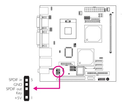
The S/PDIF connector is used to connect an external S/PDIF port. Your S/PDIF port may be mounted on a card-edge bracket. Install the card-edge bracket to an available slot at the rear of the system chassis then connect the audio cable connector to the S/PDIF connector. Make sure pin 1 of the audio cable connector is aligned with pin 1 of the S/PDIF connector.
