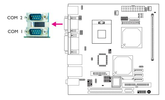
The serial ports are RS-232 asynchronous communication ports with I6C550A-compatible UARTs that can be used with modems, serial printers, remote display terminals, and other serial devices.
