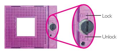
5. Position the CPU above the socket. The gold triangular mark on the CPU must align with pin I of the CPU socket.
