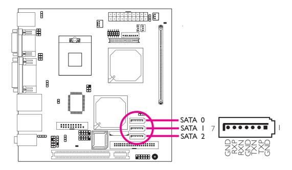
The Serial ATA ports are used to connect Serial ATA devices. Connect one end of the Serial ATA cable to a SATA port and the other end to your Serial ATA device.
