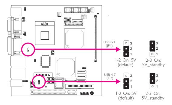
JP4 (for USB 0-3) and JP2 (for USB 4-7) are used to select the power of the USB ports. Selecting 5V\_standby will allow you to use a USB device to wake up the system. If you want to use the optional wake up function, you must enable this function in the BIOS then set the jumpers' pins 2 and 3 to 5V\_standby.
