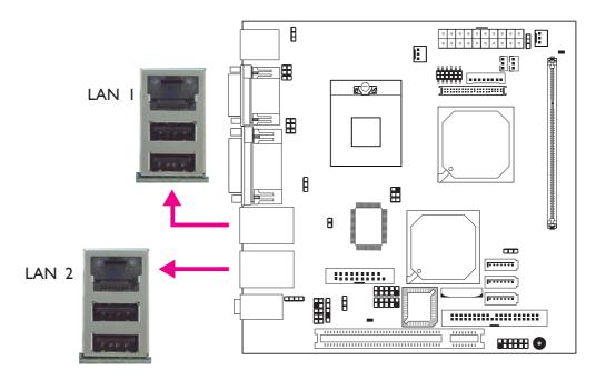
The LAN ports allow the system board to connect to a local area network by means of a network hub.
