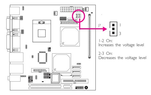
Use J7 to connect to the LCD Brightness Control button of the LCD Display Panel. It is used to adjust the brightness of the LCD Display Panel. Increasing or decreasing the voltage to control the LCD panel's brightness varies among Inverters. You must refer to the Inverter's specification to make the appropriate adjustment to the brightness of the LCD panel.
