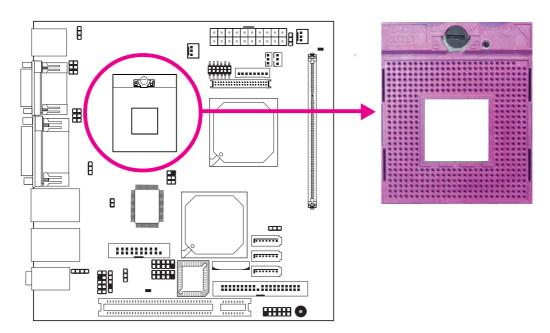
4. Use a screwdriver to turn the screw to its unlock position.
