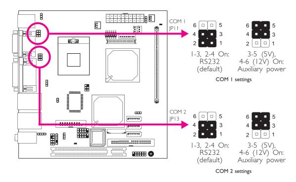
COM I and COM 2 are RS-232 ports. If the serial device connected to COM I and/or COM 2 requires 5V/12V power from the system board, set JPII and/or JPI3 pins 3-5 (5V) and 4-6 (12V) to On. Otherwise, leave the jumper's setting at I-3, 2-4 On.
