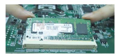
10. Push down the module until the clips at each end of the socket lock into position. You will hear a distinctive "click", indicating the module is correctly locked into position.
