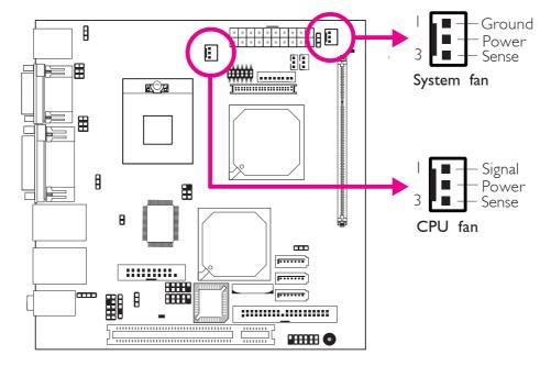
Connect the CPU fan's cable connector to the CPU fan connector on the system board. The system fan connector is used to connect an additional cooling fan. The cooling fans will provide adequate airflow throughout the chassis to prevent overheating the CPU and system board components.
