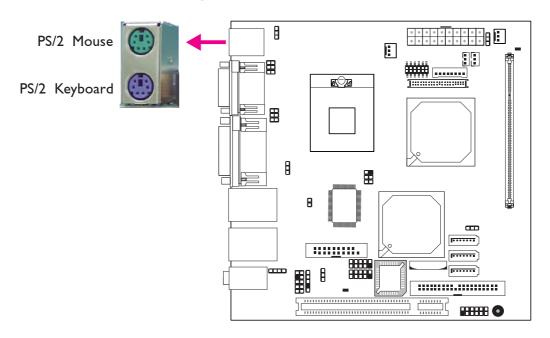
These ports are used to connect a PS/2 mouse and a PS/2 keyboard. The PS/2 mouse port uses IRQ12. If a mouse is not connected to this port, the system will reserve IRQ12 for other expansion cards.
