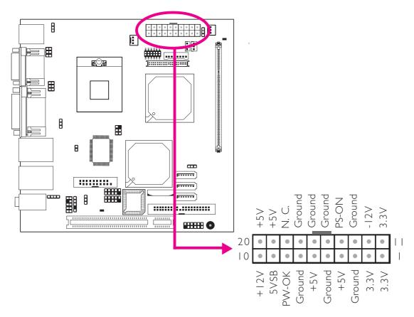
Connect a 20-pin ATX main power connector from the power supply unit to the ATX connector. The system board requires a minimum of 120 Watt power supply to operate. We recommend that you use a power supply that complies with the ATX12V Power Supply Design Guide Version 1.1.
