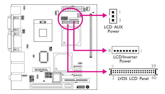
The system board allows you to connect a LCD Display Panel by means of the LVDS LCD panel connector and the LCD/Inverter power connector. These connectors transmit video signals and power from the system board to the LCD Display Panel. The LCD AUX power connector is used to connect auxiliary power to the LCD panel.
