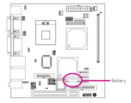
The lithium ion battery powers the real-time clock and CMOS memory. It is an auxiliary source of power when the main power is shut off.
