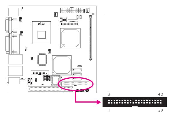
The 40-pin IDE connector is used to connect hard drives. To prevent improper IDE cable installation, the IDE connector has a keying mechanism. The connector on the IDE cable can be inserted into the connector only if pin I of the cable connector is aligned with pin I of the IDE connector.
