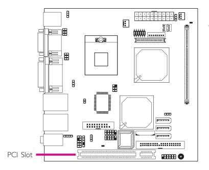
You can install a PCI expansion card or a customized riser card designed for I, 2 or 3 PCI slots expansion (for low profile PCI card only) into the PCI slot.
