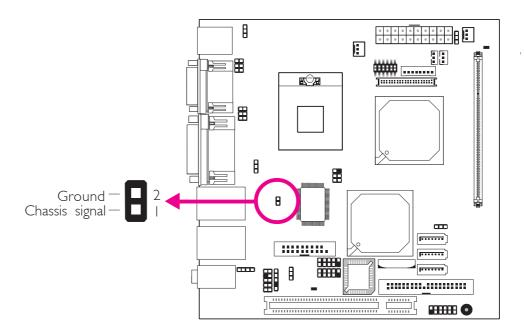
The system board supports the chassis intrusion detection function. Connect the chassis intrusion sensor cable from the chassis to the chassis intrusion connector. Whenever a chassis component has been removed, the sensor sends signal to the connector alerting you of a chassis intrusion event.
