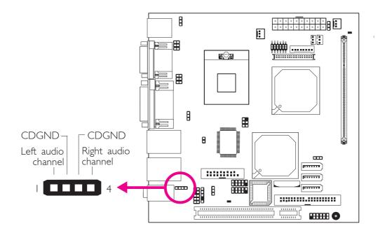
The CD-in connector is used to receive audio from a CD-ROM drive, TV tuner or MPEG card.
