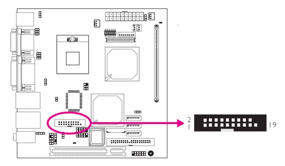
The Digital I/O connector provides powering-on function to an external device that is connected to this connector.
