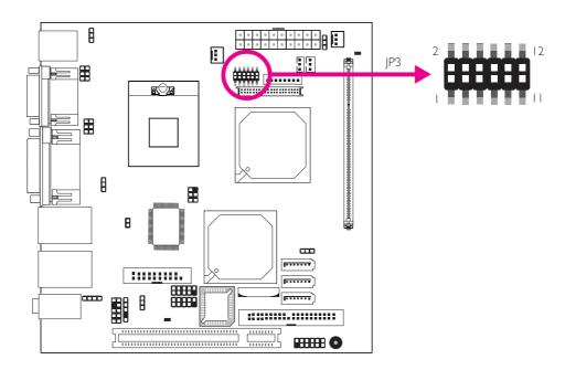
JP3 is used to select the power supplied to the LCD panel and to configure the inverter.
