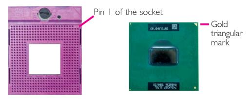
6. Insert the CPU into the socket until it is seated in place. The CPU will fit in only one orientation and can easily be inserted without exerting any force. Use a screwdriver to turn the screw to its lock position.
