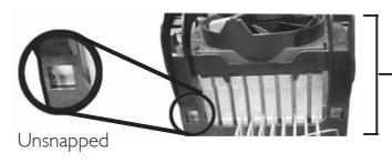
Fan / heat sink and retention mechanism assembly
