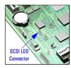
The LED cable supplies SCSI LED activity to the front panel hard disk LED. For this to work, the SCSI LED cable must be connected to the LED Activity connector on the Ultra2 SCSI PCI Adapter card (refer to graphic on page 86) and the SCSI LED connector on the system board.
