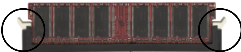
Figure 10 - DIMM module clip after installation
