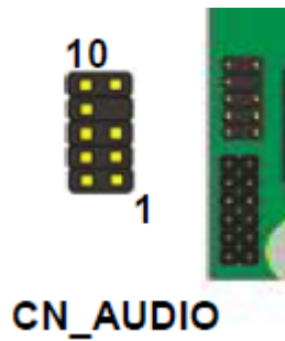
Figure 12: Audio Note Connector Type: 10-pin (5 x 2) 2.0mm-pitch header
