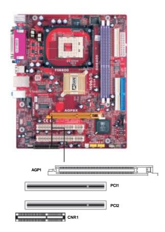
Follow the steps below to install an AGP/CNR/PCI expansion card.
