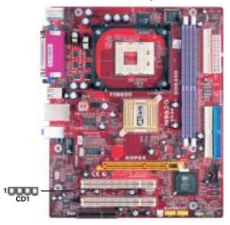
When you first start up your system, the BIOS should automatically detect your CD-ROM/DVD drive. If it doesn't, enter the Setup Utility and configure the CD-ROM/DVD drive that you have installed. On the motherboard, locate the 4-pin header **CD1**.
