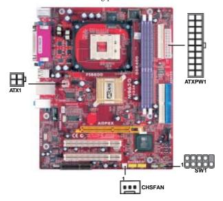
Connect the power connector from the power supply to the **ATXPW1** connector on the motherboard. The **ATX1** is a +12V connector for CPU Vcore power. If there is a cooling fan installed in the system chassis, connect the cable from the cooling fan to the **CHSFAN** fan power connector on the motherboard. Connect the case switches and indicator LEDs to the **SW1** header. Here is a list of the SW1 pin assignments.
