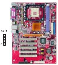
When you first start up your system, the BIOS should automatically detect your CD-ROM/DVD drive. If it doesn't, enter the Setup Utility and configure the CD-ROM/DVD drive that you have installed. On the motherboard, locate the 4-pin header CD1.
