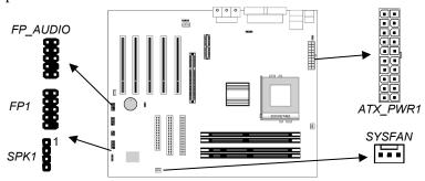
Connect the power connector from the power supply to the ATX PWR1 connector on the mainboard.
