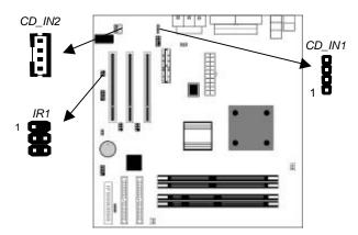
On the mainboard, locate the two 4-pin connectors **CD\_IN1** and **CD\_IN2**. There are two kinds of connectors because different brands of CD-ROM drives have different kinds of audio cable connectors. Connect the cable to the appropriate connector.
