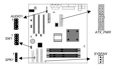
Connect the power connector from the power supply to the **ATX PWR** connector on the mainboard.
