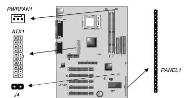
Connect the power connector from the power supply to the **ATX1** connector on the mainboard.
