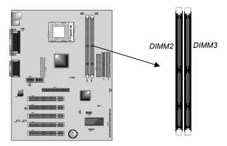
For this mainboard, you must use 168-pin, 3.3V unbuffered PC100 or PC133 SDRAM memory modules. You can install any size memory module from 32 MB to 512MB, so the maximum memory size is  $2 \times 512MB = 1GB$ .
