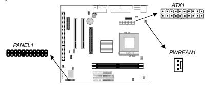
Connect the power connector from the power supply to the **ATX1** connector on the mainboard.
