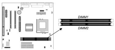
For this mainboard, you must use 168-pin, 3.3V unbuffered PC100 or PC133 SDRAM memory modules. You can install any size memory module from 16 MB to 512MB, so the maximum memory size is  $2 \times 512MB = 1GB$ .
