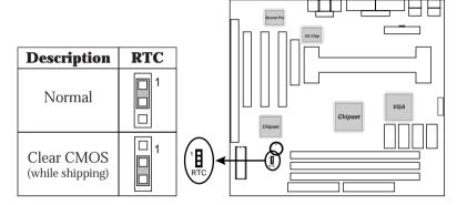
Note: 1. This jumper needs to be set on Normal Mode before using.
