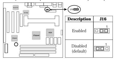
Note: Make sure that the system power can provide 800mA on +5VSB(+5V Standby) signal before using Keyboard Power On function
