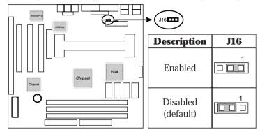
Note: Make sure that the system power can provide 800mA on +5VSB(+5V Standby) signal before using Keyboard Power On function.
