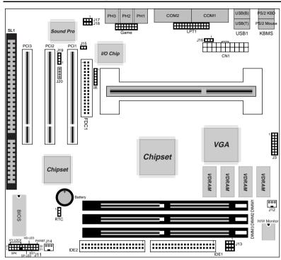
Figure 2–1. Mainboard Component Locations
