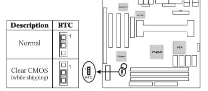
Note: 1. This jumper needs to be set on Normal Mode before using.
