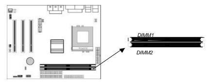
For this mainboard, you must use 168-pin, 3.3V unbuffered SDRAM memory modules. If the installed CPU uses a 100MHz system bus, you must use PC100 or PC133 memory; if a 66MHz system bus, you must use PC66 memory. You can install any size memory module from 16 MB to 512MB, so the maximum memory size is  $2 \times 512MB = 1GB$ .
