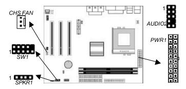
Connect the power connector from the power supply to the **PWR1** ATX Power connector on the mainboard. If there is a cooling fan installed in the system chassis, connect the cable from the cooling fan to the CHS **FAN** fan power connector on the mainboard. Connect the cable from the PC speaker to the **SPKR1** header on the mainboard.
