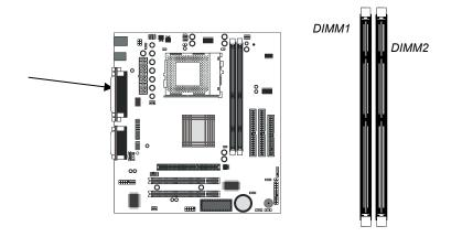
For this mainboard, you must use 168-pin, 3.3V unbuffered SDRAM memory modules. If the installed CPU uses a 100MHz system bus, you must use PC100 or PC133 memory. If the installed CPU uses a 66MHz system bus, you must use PC66 memory. You can install any size memory module from 16 MB to 512MB, so the maximum memory size is  $2 \times 512MB = 1GB$ .
