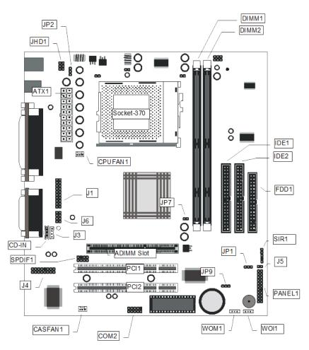
**Note:** Any jumpers on your mainboard that do not appear in this illustration are for testing only.
