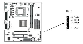
1. Locate the infrared port SIR1 header on the mainboard.
