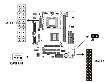
Connect the power connector from the power supply to the ATX1 connector on the mainboard.
