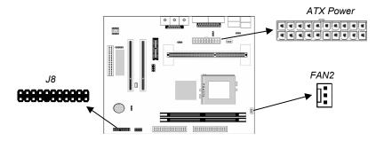
Connect the power connector from the power supply to the **ATX** Power connector on the mainboard.
