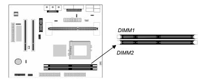
For this mainboard, you must use 168-pin, 3.3V unbuffered SDRAM memory modules. If the installed CPU uses a 100MHz system bus, you must use PC100 or PC133 memory. If the installed CPU uses a 66MHz system bus, you must use PC66 memory. You can install any size memory module from 16 MB to 512MB, so the maximum memory size is  $2 \times 512MB = 1GB$ .
