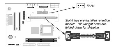
2. The Slot-1 is installed with a retention module. The upright arms of the module are folded down for shipping. Raise the arms so that they are in the upright position.
