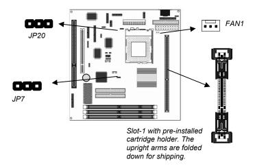
2. The Slot-1 is installed with a cartridge holder. The upright struts of the cartridge holder are folded down for shipping. Pull the struts upwards so that they are in the upright position.
