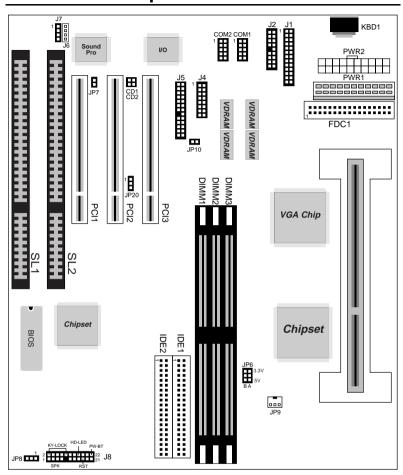
Figure 2–1. Mainboard Component Locations
