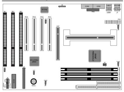
Figure 2–1. Mainboard Component Locations
