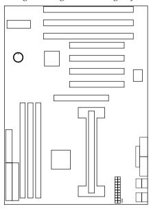
Insert the 2 pairs of screws (1a or 1b, depending on the type you received) from the bottom of the motherboard upward onto the mainboard.
