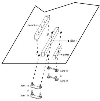
Insert the 2 latches into the two holes of the supporting base and then turn them 90° to secure the CPU.
