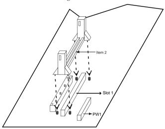
If the retention clip is installed incorrectly, you will not be able to insert the CPU into the retention clip and in this situation you might need to rotate the retention clip by  $180^{\circ}$ .
