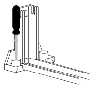
And for 1b and 2b retention mechanism, simply push the latches in to secure the screws.
