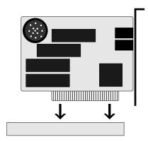
Figure 3-5: Installing a Plug & Play Card
