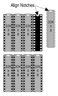
Figure 3-2: Upgrading the External Cache
