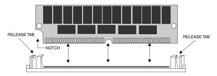
Figure 3-1: Installing a 72-Pin SIMM
