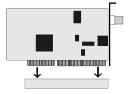
Figure 3-4: Installing an EISA Card
