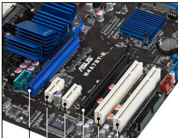
Primary PCI Express x16_1 slot (blue, at max. x16 link) PCI Express x1_1 slot PCI Express x1_2 slot PCI_1 slot PCI_2 slot PCI Express x 16_2 slot (black, at max. x8 link)
