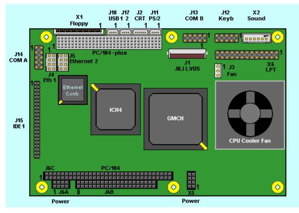
Notes: The position of Pin 1 is marked with a quadratic pad on the PCB.
