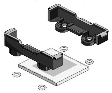
2) Insert Black securing peg into bracket holes
