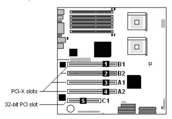
PCI slots A1, A2, B1 and B2 are all PCI-X slots while PCI slot C is a conventional 32-bit/33MHz PCI slot. However, PCI slots A1, A2, B1 and B2 will operate at the speed of the slowest PCI card that is installed into them. If a 33MHz PCI card is inserted into bus A, both A slots will operate at 33MHz. The same rule applies for Bus B slots. **A1 and A2 are BUS-A** and **B1 and B2 are BUS-B**.
