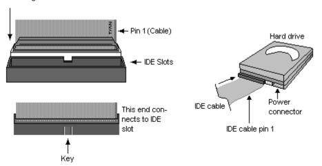
Simply plug in the BLUE END of the IDE cable into the motherboard IDE connector, and the other ends into the drive(s). Each standard IDE cable has three connectors, two being close to each other. The BLUE connector that is far on its own is the end that plugs into the motherboard whereas the other two connectors are used to connect to drives.
