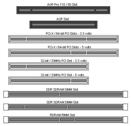
Simply find the appropriate slot for your expansion card and insert the card firmly. Do not force any expansion cards (or anything else) into any slots if they refuse to go in. It is better to try another slot or return the faulty card rather than damaging both the motherboard and the card.
