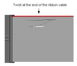
The first floppy drive (sometimes denoted as **A:**) is usually attached to the end of the cable with the twist in it. Drive B: is usually connected to the second or third connector in the cable (the second or third connector after you install Drive **A:**).
