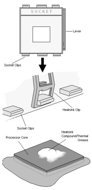
First, use thermal compound (also called heatsink compound or thermal grease) and apply a small amount on to the processor's core – the small shiny square in the center of the processor.
