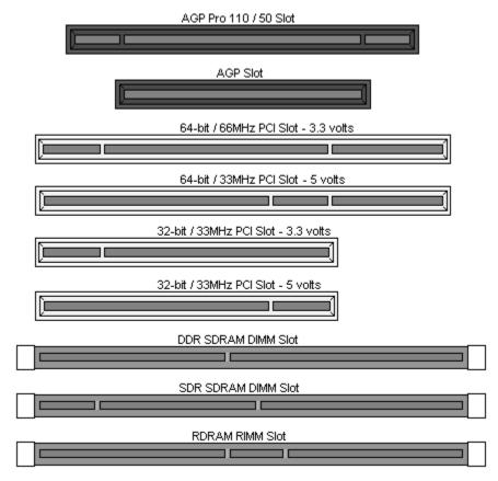
Simply find the appropriate slot for your expansion card and insert the card in firmly. Do not force any expansion cards (or anything else) into any slots if they refuse to go in. It's better to try another slot or return the faulty card rather than damaging both the motherboard and the card.
