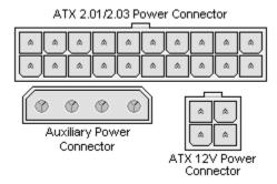
By utilizing an Auxiliary drive power connector, you can use virtually any existing ATX 2.01/2.03 standard power supply to operate the Tiger MPX. Simply attach the connectors and proceed forward. Also, it is not necessary to connect all three and there is no harm in doing so.
