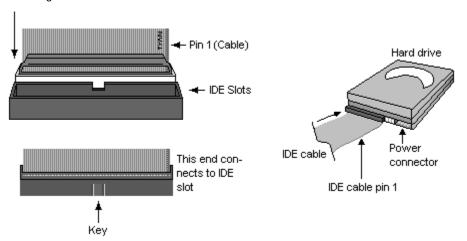
Simply plug in one end of the IDE cable into the IDE connector and the other ends into the drive(s). Each standard IDE cable has three connectors, two being close to each other. The connector that is far on its own is the end that plugs into the motherboard whereas the other two connectors are used to connect to drives.
