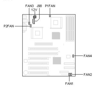
FANs 1 to 4 are used for chassis cooling while P1FAN and P2FAN are used to attach processor fans. To ensure safe and reliable operation, do not mix and match chassis fans connectors with the P1FAN/P2FAN connectors.
