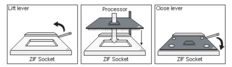
The processor you choose to use may not look exactly like the one pictured above, nor will the socket look exactly the same. For example, your processor may appear to be in a different color and have different markings on it. The diagram is provided as a visual guide to help you install the processor.
