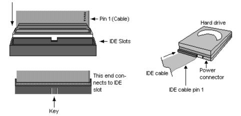
Attaching IDE cables to the IDE connectors is illustrated below:
