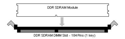
Once the memory modules are firmly seated in the socket, two clamps on either side will close and secure the module into the socket. Sometimes you may need to close the clamps manually.
