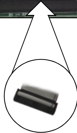
Match striped side with Pin 1
