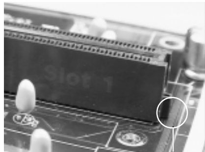
Pentium II Slot Connector and Key Pin
