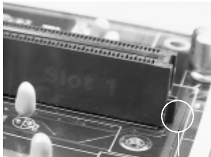
Figure 14 Pentium II Slot Connector and Key Pin
