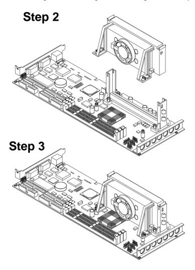
Figure 1-6: Mounting CPU and cooling modules - Step 3
