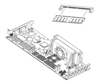
Figure 1-3: DIMM installation
