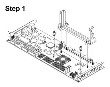
Figure 1-4: Mounting CPU and cooling modules - Step 1
