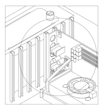
Figure 1-7: On-board support bracket
